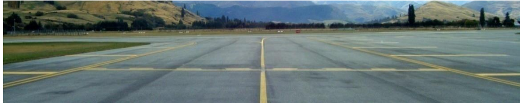
16-4 - Runway Hold Point Marking – Alpha 3
