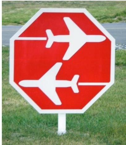
16-14 - Stop Sign (Taxiway Crossing)
